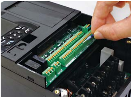
Screwless terminal block (control terminal block).
